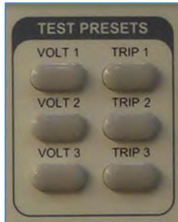
Figure 4-7: TEST PRESET keys for Test Setups 1 through 3
