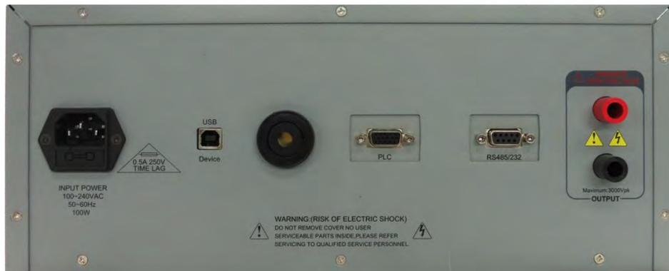
Figure 4-5: 1657 Rear Panel Connector Locations (shown with optional RS232, PLC Interface and -RPC)
